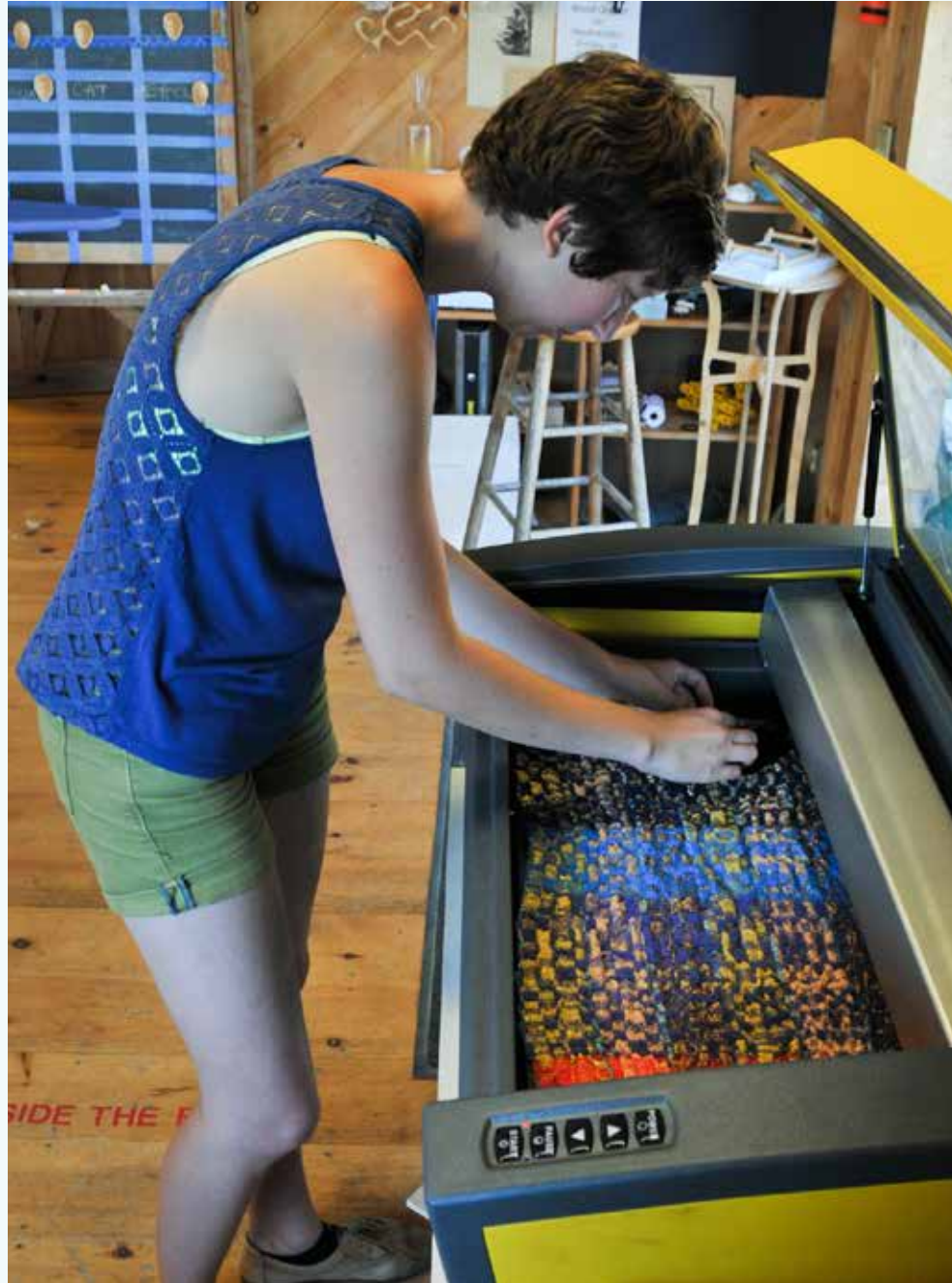
FIG. 2 A student at Haystack Mountain School of Crafts in Deer Isle, Maine, cuts vinyl on a laser cutter in the school's digital fabrication laboratory (fab lab).
